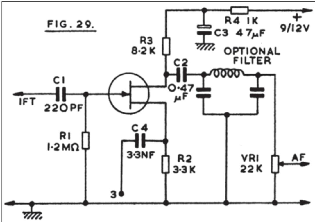
Two inputs are required to the FET. That to C1 is taken from the secondary of the final IFT in the receiver. C4 is connected to 3 in Figure 28.
