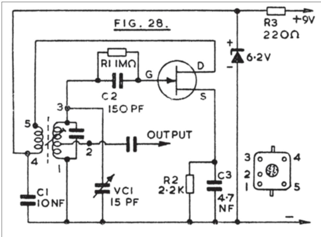
A control knob is necessary on VC1, as this must be adjustable during reception. If it is not practical to include this control on the receiver, then the BFO can be constructed as a separate unit.
