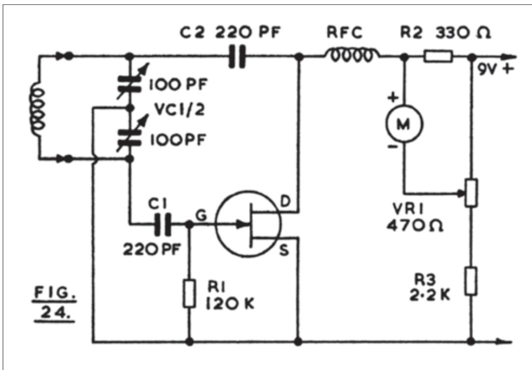
Due to the bridge circuit and fact that this is controlled by the drain current, the change present to operate the meter is much larger than in Figure 23, and it will be found that a 1mA instrument can be fitted. With a very sensitive meter, readings can tend to go off the scale too easily, so that frequent adjustment of VR1 is needed.
