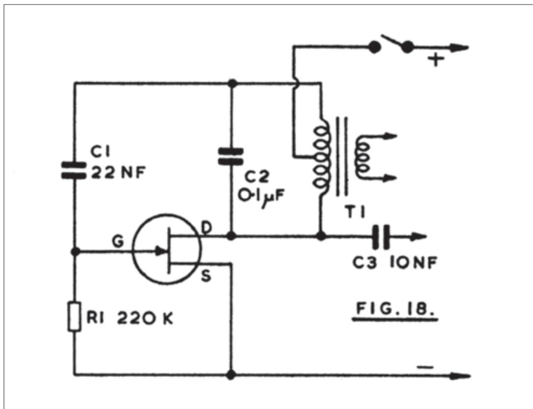
Tone and output can be altered by changing any of the component values, or by including a source resistor of 1k to 2.7k or so.
