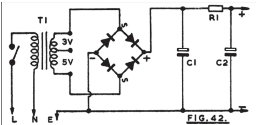
Figure 42 is the circuit of a power supply which can be used for any item requiring approximately  $4\frac{1}{2}$ v to 12v.
