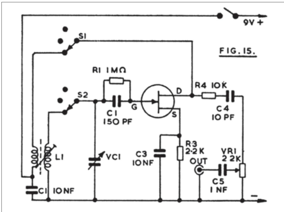
for each range is as shown below, which indicates the bands over which these coils can be used, with a capacitance swing of approximately 20-350pF for VC1.
