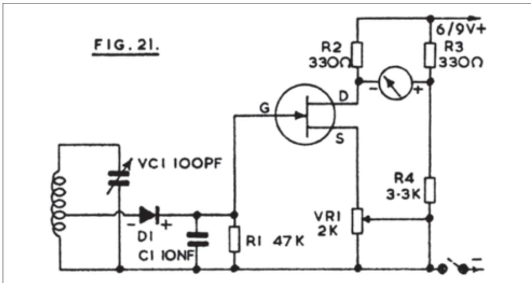
tion, VC1 tunes the inductor to resonance so that D1 produces a positive voltage across R1, for the FET gate. The meter itself is in a bridge circuit, VR1, the FET and R2 being one side, and R3/R4 the other side. Balance, or zero current through the meter, is obtained by setting VR1. Balance is then upset when the gate moves positive, and the indication can be half scale or more, so that good sensitivity is obtained.
