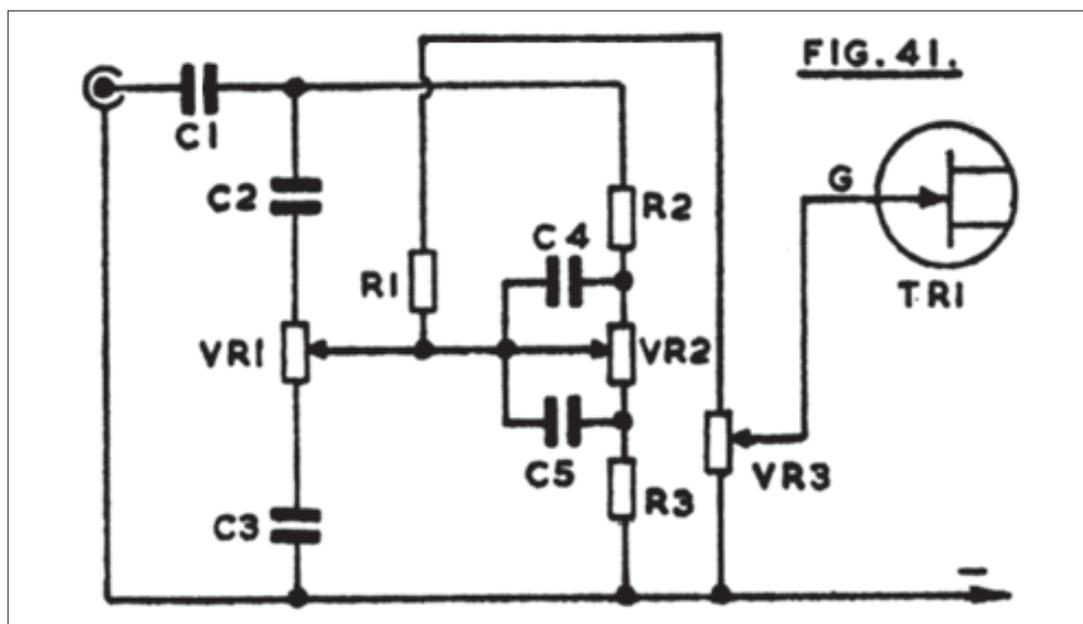
C1 is the input isolating capacitor, and may be unnecessary with some types of input. VR1 is for treble control. Treble is lifted with the wiper towards C2, whose reactance falls as frequency rises. With VR1 wiper towards C3, treble is reduced. VR2 similarly provides lift or cut in bass. Both are linear controls, supplying the volume control VR3 by means of R1. The source and drain circuits for the FET can be as in Figure 40.
