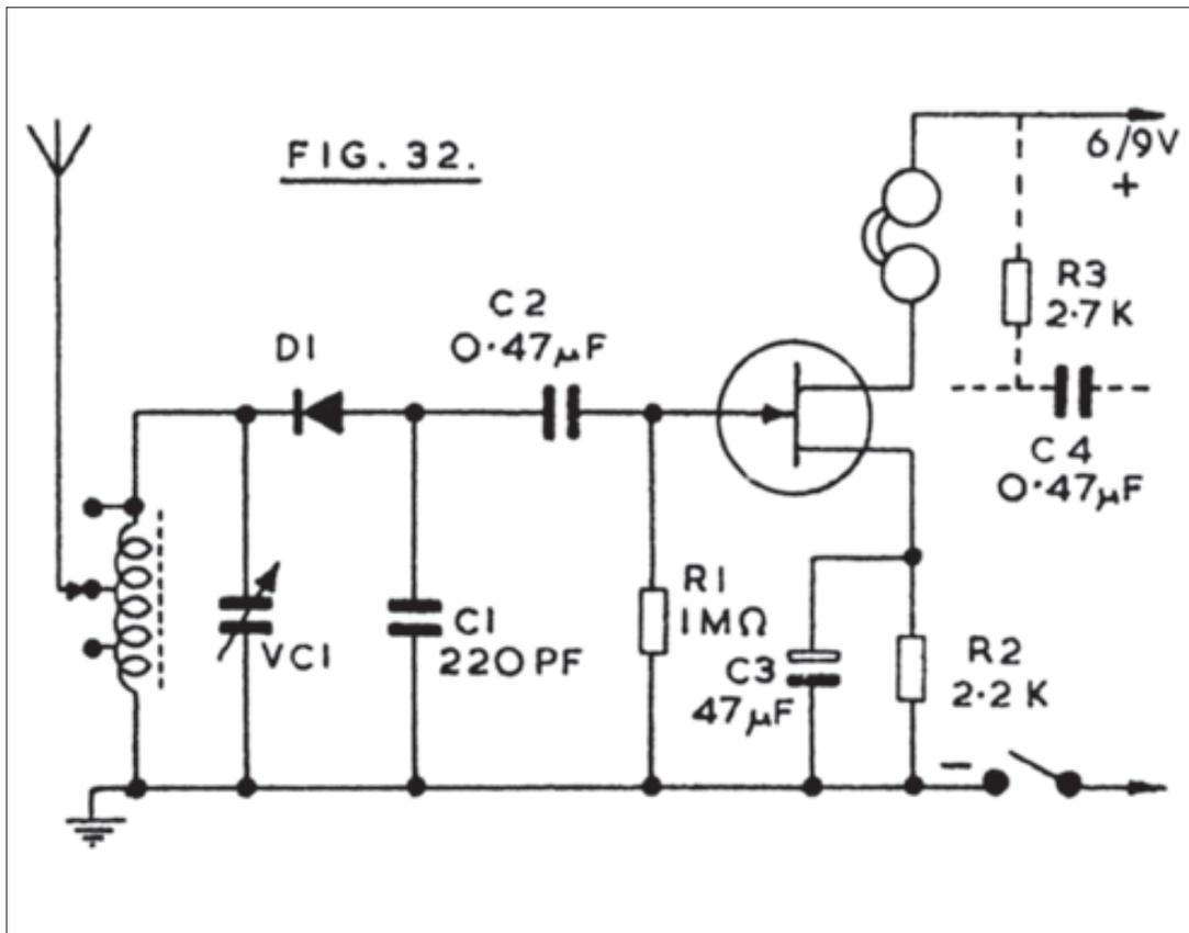
For other than short aerials, it is useful to have tapings, as in Figure 32, to allow sharper tuning. These taps may be at about the middle of the winding, and one quarter the total number of turns from the earthed end. Some coils may have a primary, or aerial coupling winding, which can be used instead.
