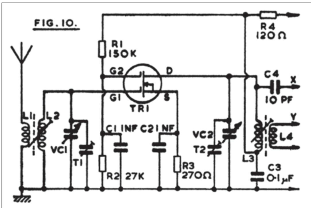
side by side on a 7mm cored former. With a 2-gang 100pF capacitor for VC1/VC2, coverage is approximately 11 to 32MHz. Trimmer T1 and T2 can each be 20pF.
