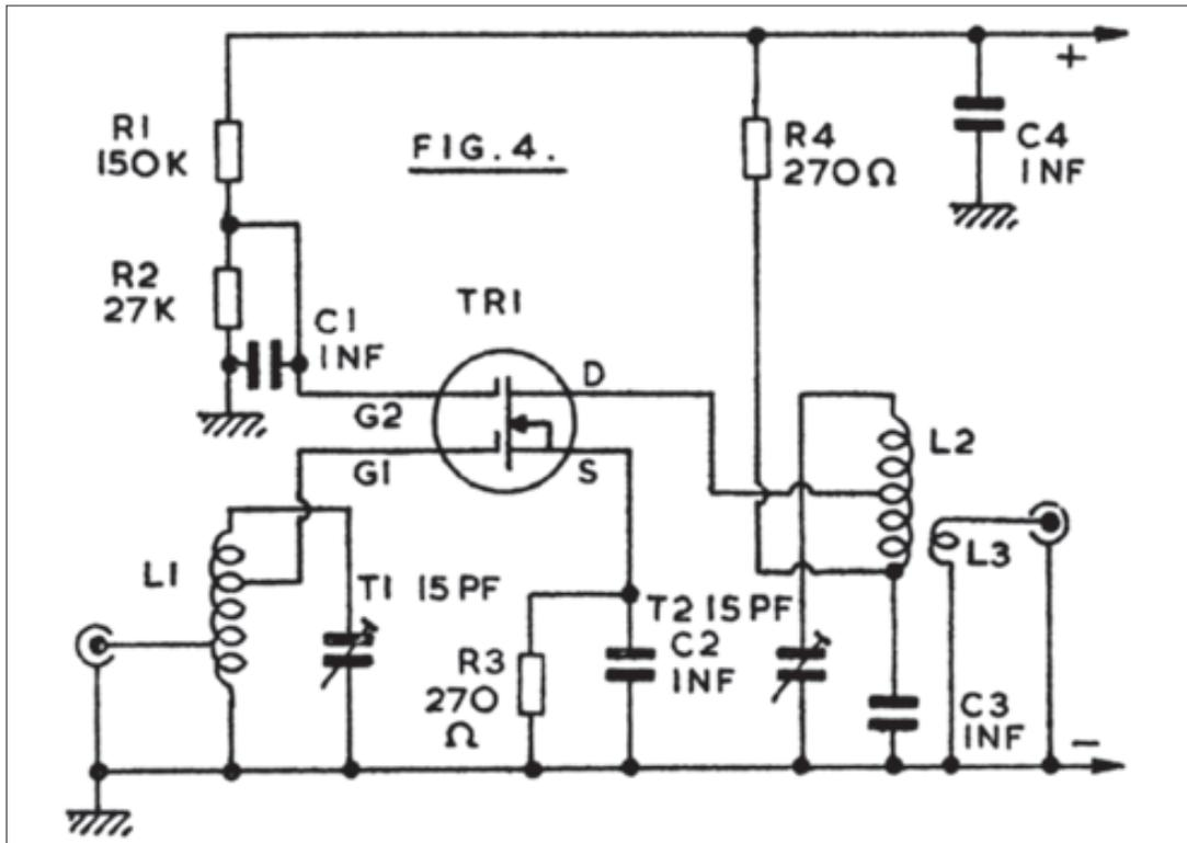
take L1 and L2. A small aluminium box will house the amplifier, and this allows the co-axial aerial and output sockets to be mounted as shown.
