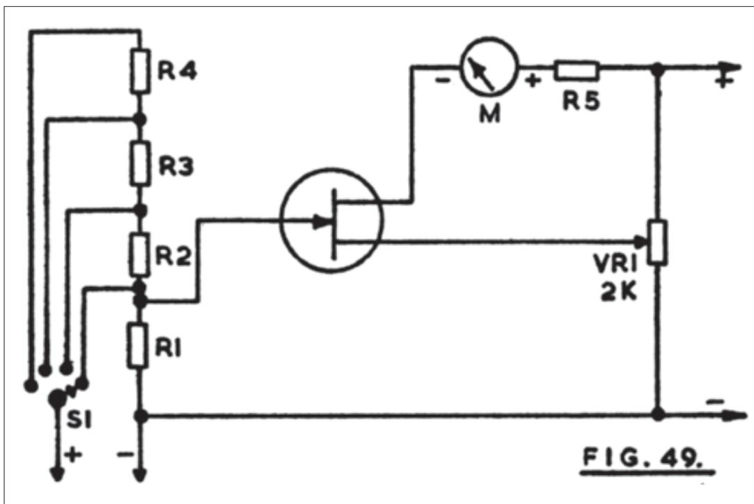
With no external voltage present, R1 maintains the gate of the FET at negative, and VR1 is set so that source current through the meter M is negligible. When the gate is made positive, M shows the source current. R5 is merely a limiting resistor, to protect the meter.
